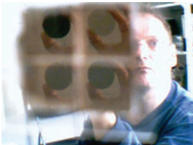
Fig. 13. A round polarizer seen through a faceted prism with polarizer mask. The total prism's size is 2.5 \text{ cm}^2 . The slopes of the prisms are set to 10^\circ slightly off the body diagonals to represent the correct camera image aspect ratio (1.333). The multiplexed images of the round polarizer are different for each facet depending on the directions of the individual polarizers in the mask for each prism section.
